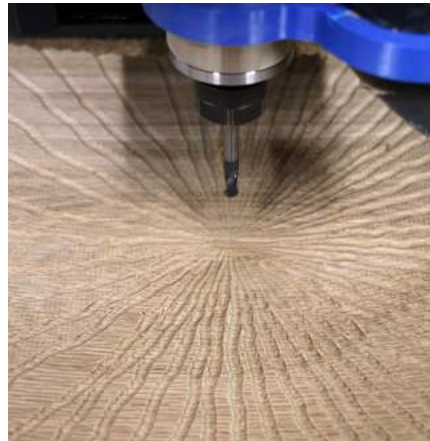
Milling machine accurately reproducing hand drawn lines.
