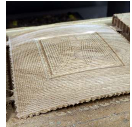
Underside of dish with milled surface pattern.
