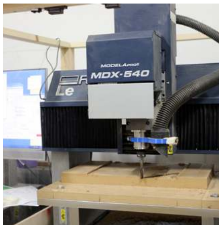
Three axis CNC milling machine used for all production.
