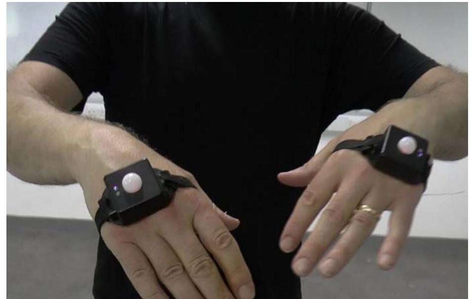
Below: Infrared trackers used by the GAMS tracking system.
