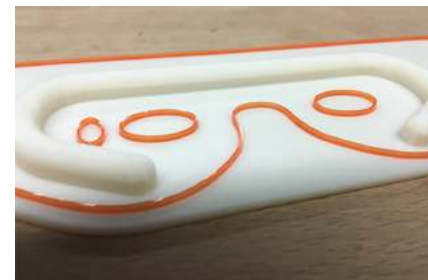
Below left: Male 'horseshoe' mould to heat press the face side of mask
