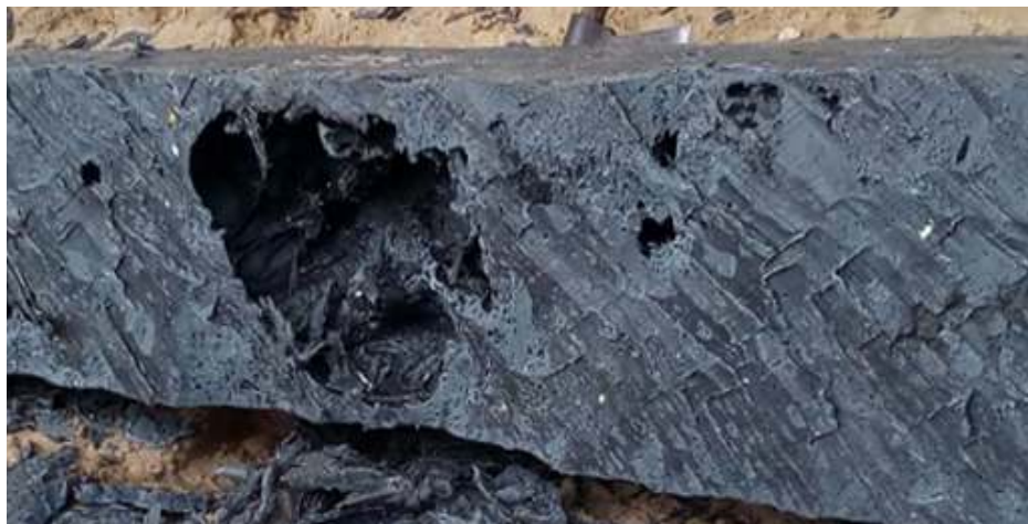
Below: Low quality recycled plastic with air bubbles. Photo Credit: Simon Scott-Harden
